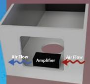
Remove coin box and replace it with the amplifier resting as shown, for safety. DO NOT use a mounting bracket to mount
